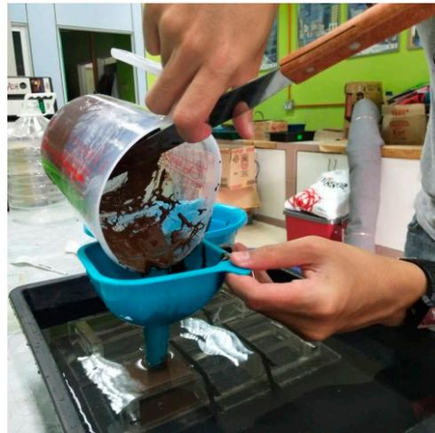
**Figure 1.** AAFA paste poured into mould in seawater.
