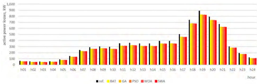
Figure 24. Hourly active power losses in the IEEE 33-bus system, for each algorithm.
