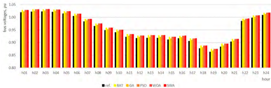
Figure 28. Voltage improvement after compensation for bus 215, low voltage, the 215-bus network.
