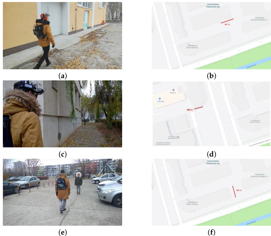
Figure 5. Examples of testing scene set ups for mobility tests in semi-controlled environments: (a) Walking by a wall (30 m path), static obstacles on the path (MT I-1); (b) Geolocation of MT I-1 testing scenario; (c) Walking by a wall (15 m path), hanging obstacles on the path (MT I-2); (d) Geolocation of MT I-2 testing scenario; (e) Walking in a parking lot (25 m path), parked cars, dynamic obstacles on the path (MT I-3); (f) Geolocation of MT I-3 testing scenario.
