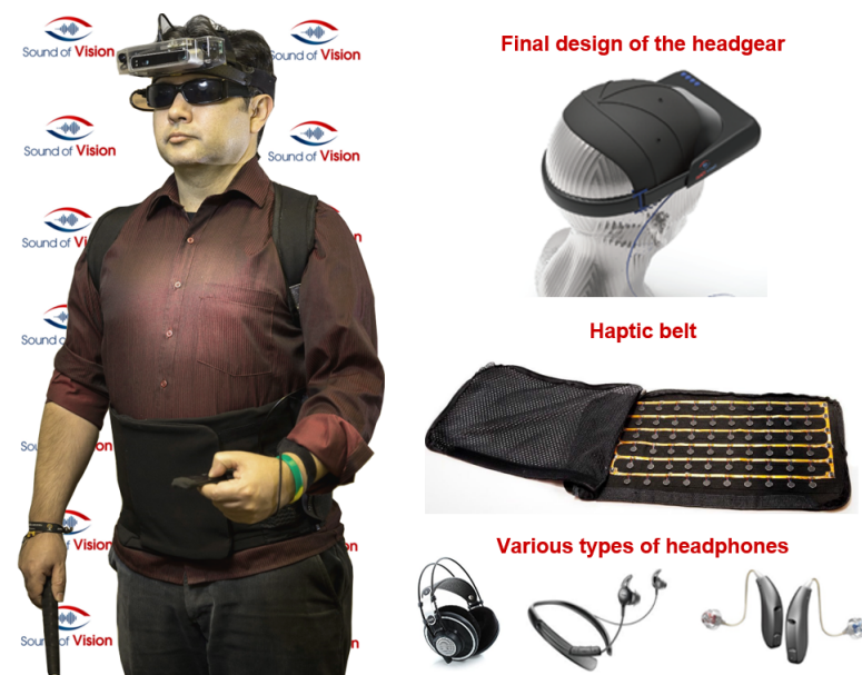
Figure 1. The Sound of Vision system. (Left) The prototype used in the usability evaluations. (Right) Various parts of the system.
