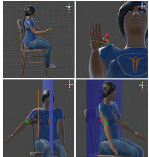
FIGURE 4. The angles considered for evaluating the movement score for Forearm Flexion-Extension (top-left), Thumb Opposition (top-right), Arm Adduction-Abduction (bottom-left), Arm Anteduction-Retroduction (bottom-right).
