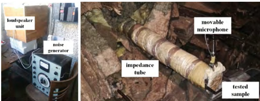
Fig. 2. Sound absorption coefficient experimental setup (according to ISO 10534-1:1998).
