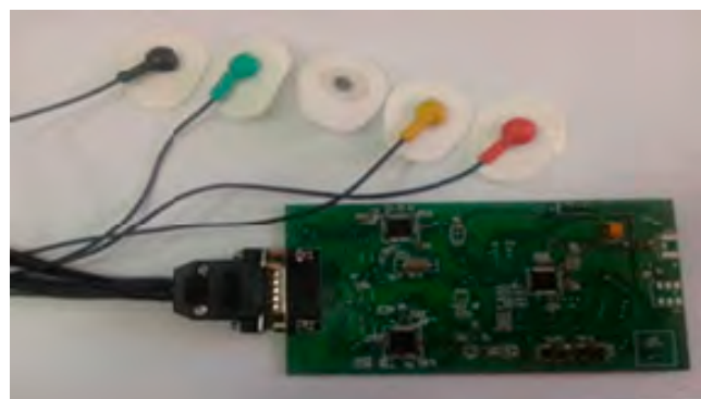
Figure 6. Experimental model using an ADAS1000 demo-board.
