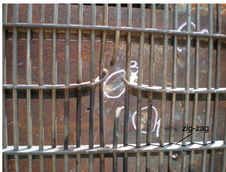
Figure 2. Patented wires in a zig-zagged configuration useful in causing projectile yaw. Zig-zag configuration of patented wires is indicated by a broken black line [15].
