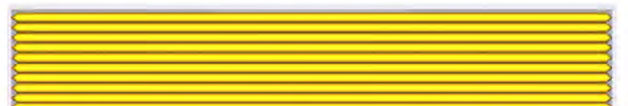
Figure 14. A 0.33 mm layer thickness 3D-printed specimen.
