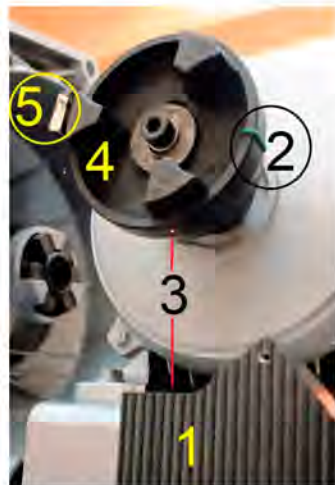
Figure 3. A view of the jaw coupling hub placed on the motor rotor.
