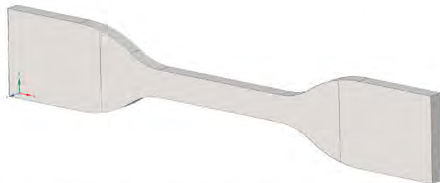
Figure 25. Screenshot of the geometry used in finite element analysis.
