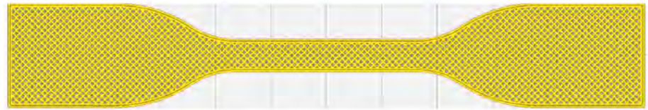
Figure 10. A 100% infill percentage 3D-printed specimen.
