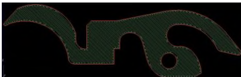
Figure 2. View of the tool paths used for 3D printing
