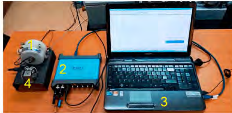
Figure 2. A view on transformers ICT (1) and IVT (4) on digital oscilloscope (2) and personal computer (3).
