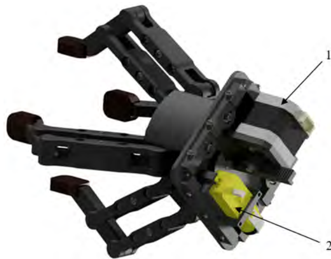
Figure 4. The electrical drive part of the gripper (1—main electric motor, 2—second electric motor).
