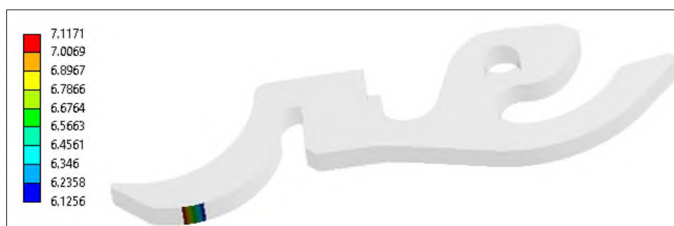
Figure 14. FEA displacement results in the measuring area for a modulus of 1.8 GPa
