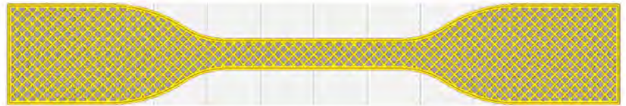
Figure 11. A 45° raster angle 3D-printed specimen.
