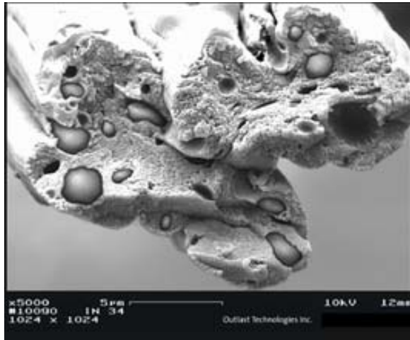
FIGURE 1. Outlast ® Thermocules ® in viscose fiber [9](with © Outlast Technologies, Inc. permission).
