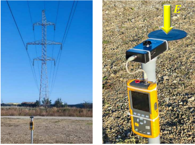
Fig. 4. Electric field measurements under the 110-kV OPL.
