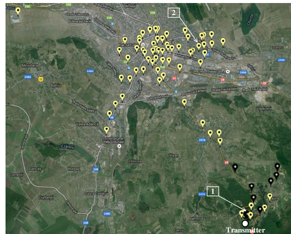
Fig. 2. Indication of the measurement locations on the map (yellow marker: E < 0.1 V/m; black marker: E > 0.1 V/m)
