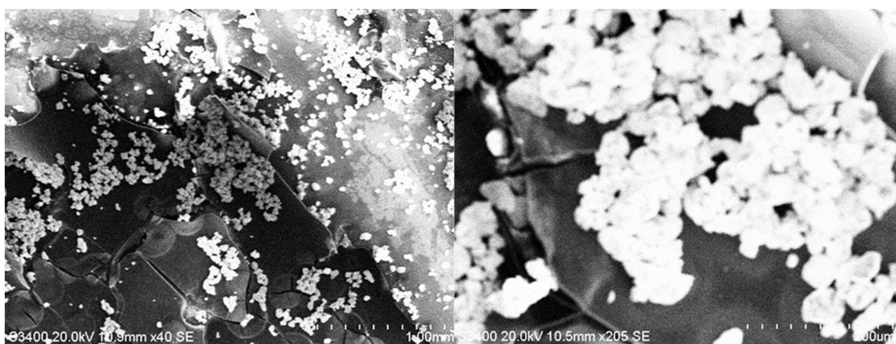
Figure 11. SEM images of \text{Al}_2\text{O}_3/\text{PEDOT:PSS} composites with Au.
