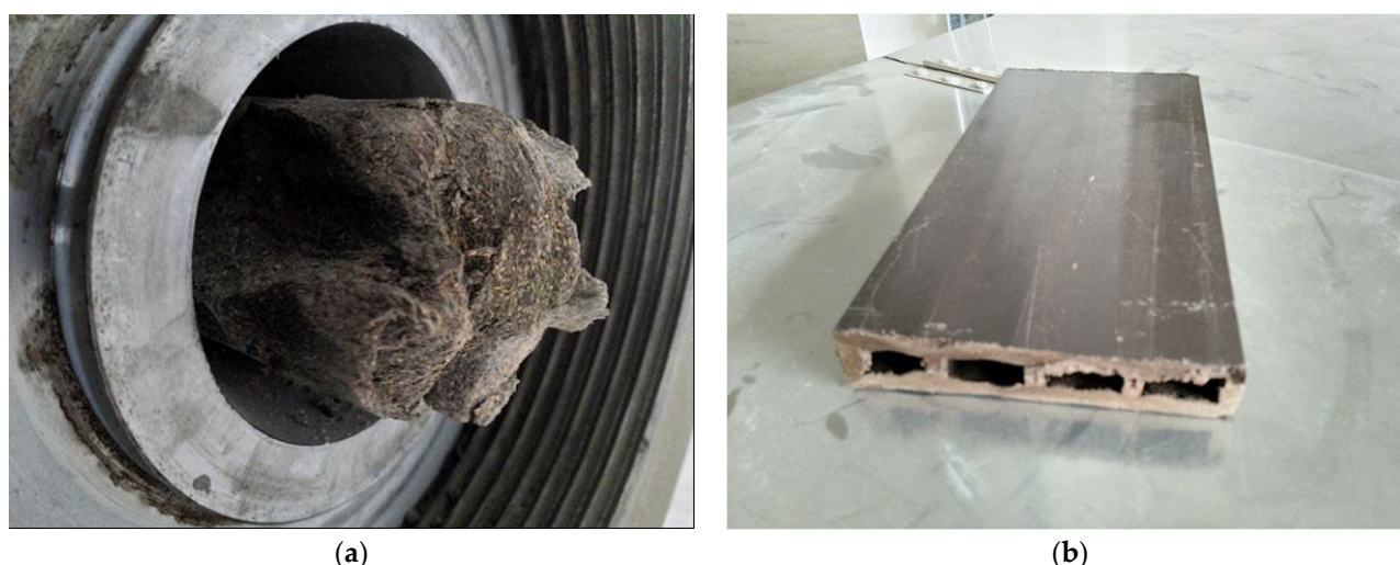
Figure 4. Thermoplastic building material. (a) Composite semi-finished material, before passing through the mold. (b) Example of profile obtained from the extrusion equipment.
