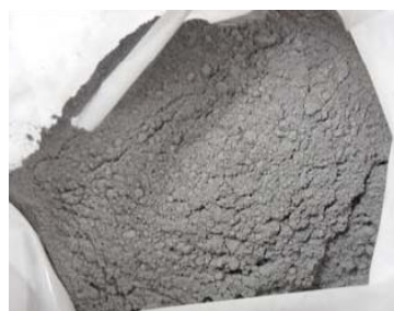
Figure 2. Image of non-metallic powder/fraction with particle size of up to 10 microns.
