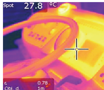
Figure 6: Temperature measured with a thermal-imaging camera on the driver's cabin
