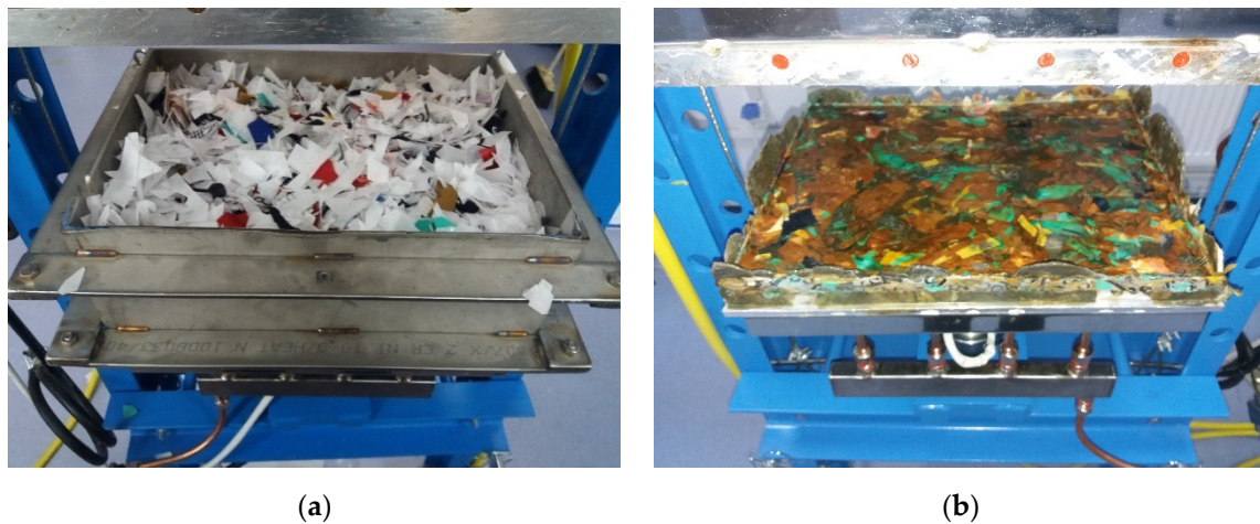
Figure 4. The waste-based composite materials panels: (a) pre-and (b) post-the technological thermoforming process.
