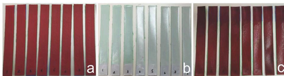
Figure 8. Complete T-peel specimen sets ( n = 8 per polymer): (a) PLA, (b) PETG, (c) TPU.
