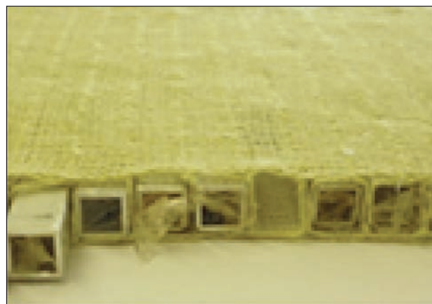
Fig. 2. U shaped sandwich knitted fabric
