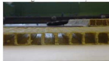
Fig. 5. Manufacturing of composite materials with 3D textile reinforcements.
