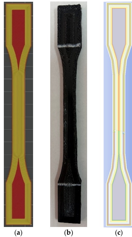
Figure 4. Specimen model: (a) plot of 3D printing process manipulation; (b) 3D intermediate printed sample made of ABS; and (c) 3D CAD model replica of the wall infill pattern.
