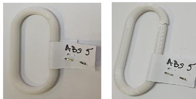
Figure 9. The appearance of a chain link made of ABS polymer material before (left) and after (right) breaking, respectively.
