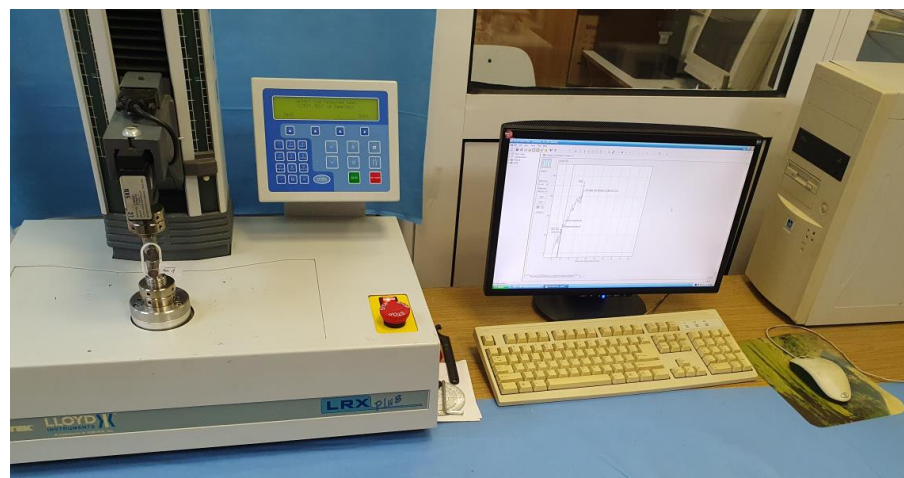
Figure 6. Components of equipment used for tensile testing of chain links.
