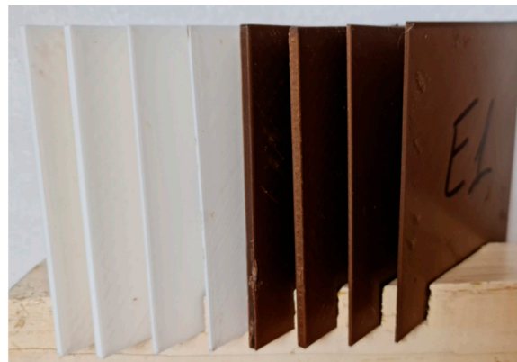
Figure 6. Test samples obtained by 3D printing of ABS (white) and PLA (brown) used to evaluate the temperature decrease in a certain time interval.
