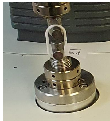
Figure 7. Clamping the chain link on the tensile testing machine.
