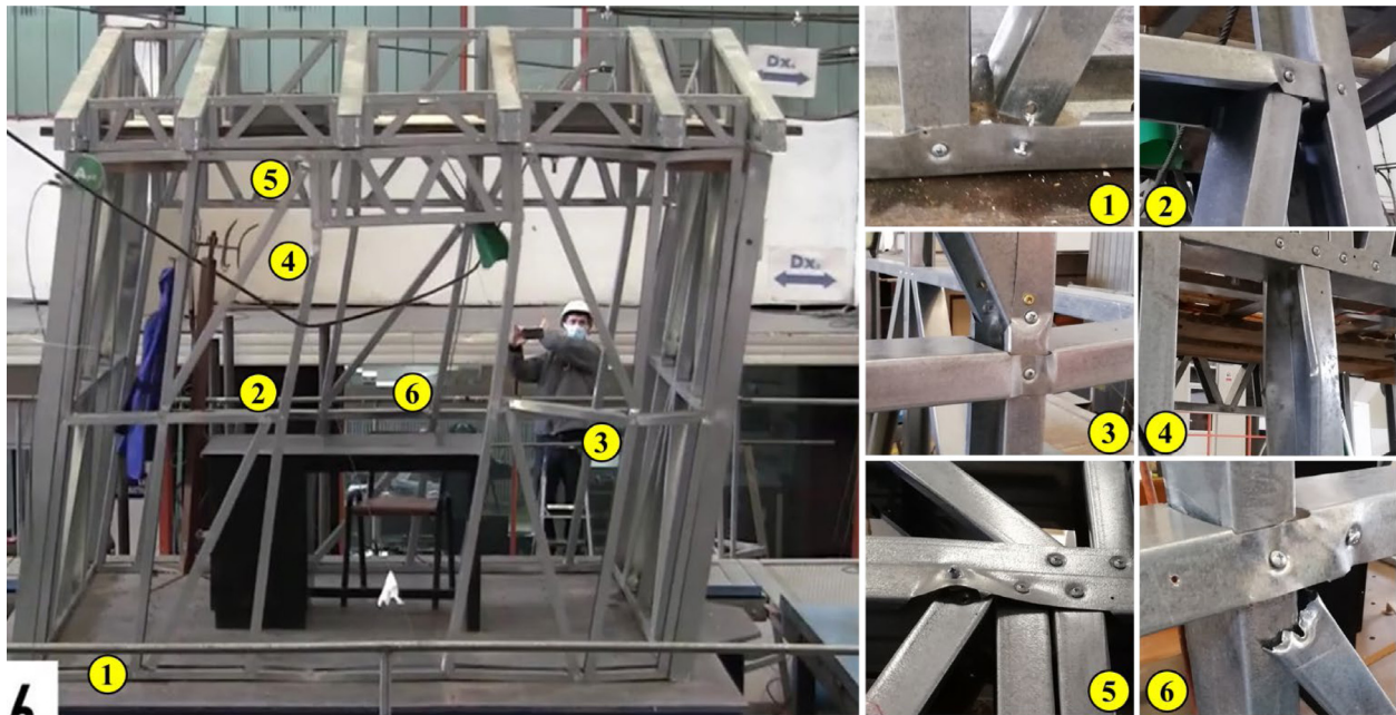
Fig. 19. Failure details mechanisms captured from video recording of the experiment.
