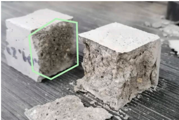
Fig. 6. Cross-section of nanomaterial-modified cement mortar sample after testing.
