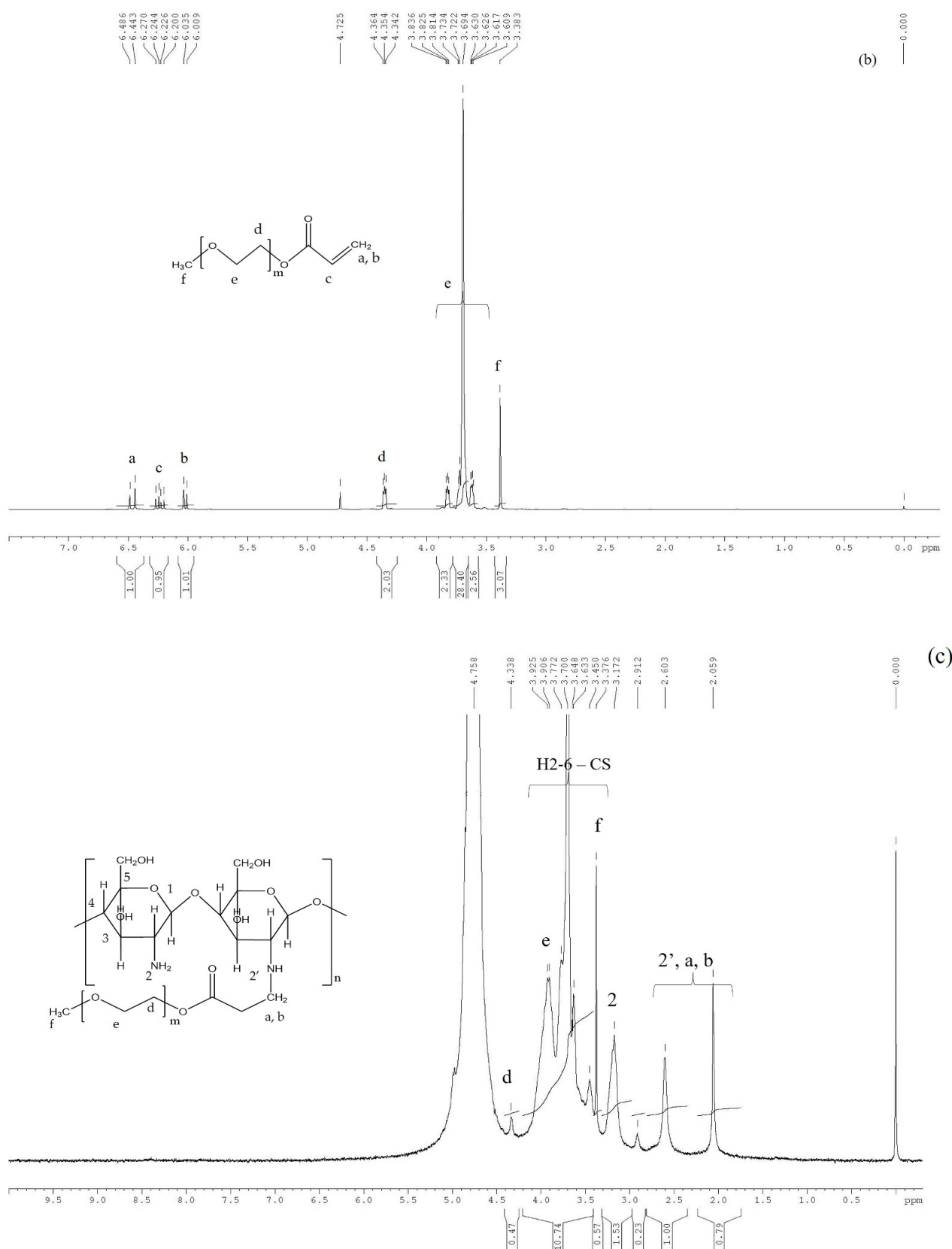
Figure 2. ^1\text{H} RMN spectra of (a) CS; (b) PEGA; (c) CS-PEGA.
